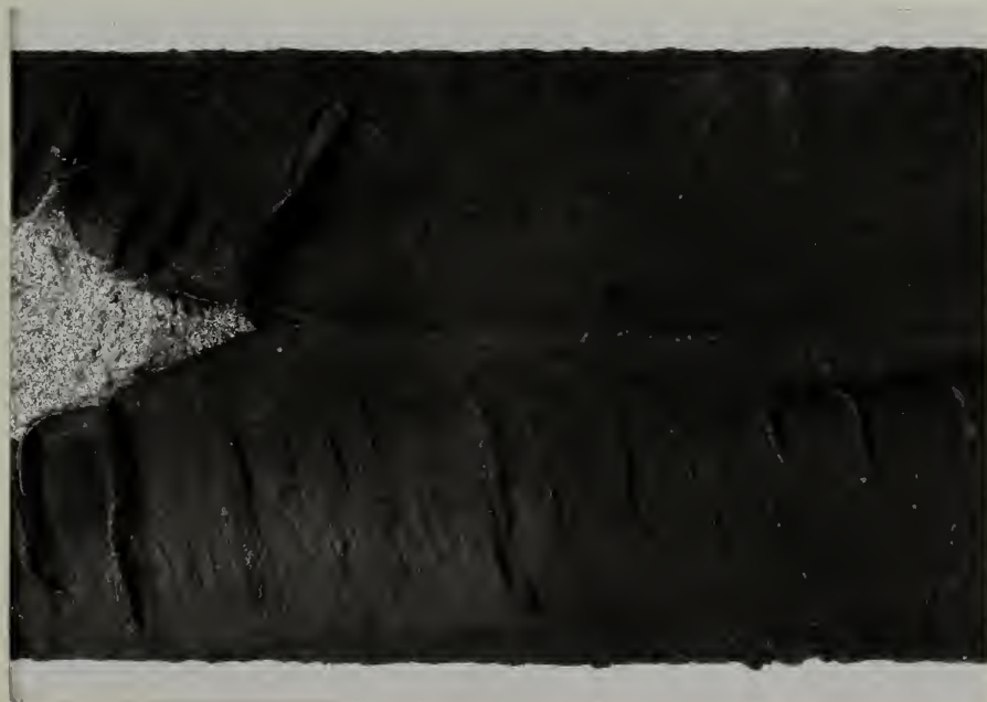
Figure 5. Fracture surface of vane 4. Upstream end is beyond right side of picture. X 3
